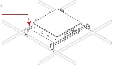
Finialize installation by adjusting height of fixture and then fully tightening wingnuts on side.
