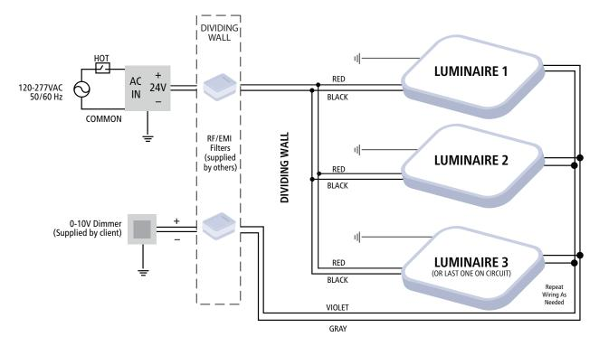
NOTE: ALL WIRES WITHIN MRI ROOM TO BE INSIDE GROUNDED RIDGID ALUMINUM CONDUIT
