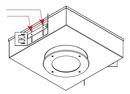
Place fixture in grid ceiling and secure by utilizing T-Grid mounting Bars (supplied by others).
