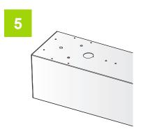
7/8" knockout is located on the back of the fixture to allow for wiring. Bring wiring through.
