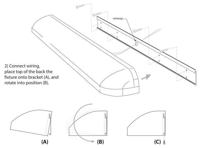
3) Using included set-screws, lock fixture into place (C). The number of set-screws will vary by fixture length.
