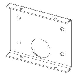
Step 2: Attach the piece with one flat end and prongs to the fixture using 4 fasteners. This allows the piece attached to the fixture to slip over and through the piece attached to the wall, as seen below.
