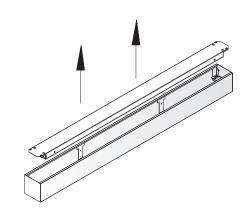
Remove LED assembly and set aside.
