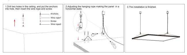
Note: 2\*2ft: 2 pcs suspension kits needed for installation. 1\*4ft: 3pcs supsention kits needed for installation.
