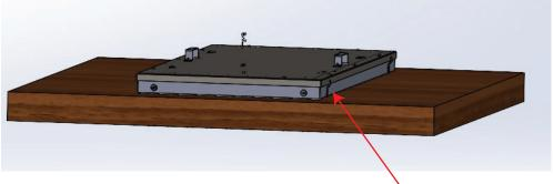
7. You have 4 optional support clips on the upper unit. These are provided to offer additional static support to secure unit to overhead structure.
