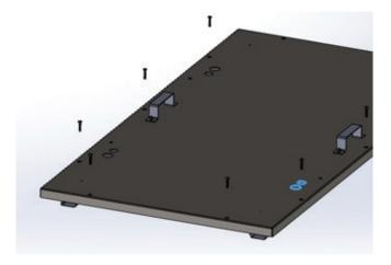
6. Re-install top plate to upper unit using screws removed from step 2.
