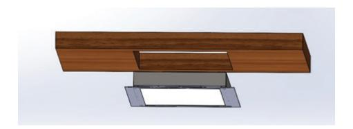
4. From the ceiling side place the upper unit into the ceiling cut out. Aligning 16 each  $#10-32 \times \frac{1}{2}$ " phillips pan head screws with the cage-nuts in the lower unit. Secure screws snug, but do not over torque.
