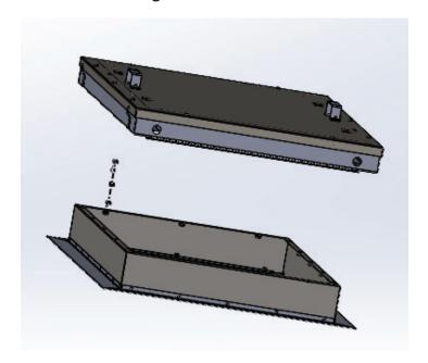
2. Locate upper unit and remove top plate 10 each  $#10-32 \times 1"$  phillips pan head screws with O-rings and secure for re-installation.
