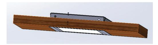
5. Locate top plate and prepare electrical connection into the optional knock outs on the top side of the electrical plate. Options are for  $\frac{1}{2}$  and or  $\frac{3}{4}$  connection.
