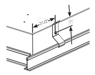
Attach mounting clips as shown, 3 1/2" from each side, and 1" from the top.
