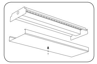
**6** Replace the driver cover. Install the lens over the housing and make sure it snaps in place securely.
