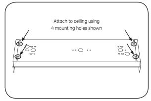
4 Use the four existing holes in the housing to drill four fasteners (optimal for the type of ceiling present) directly into the ceiling, one fastener in each hole. This fixture may be mounted directly to the junction box if desired. Each fastener should be rated to hold at least 11 pounds.
