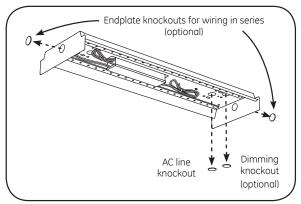
**3** Remove knockout for the AC line input wires. Optionally, remove additional knockouts for dimming wires and/or wiring adjacent fixtures in series.
