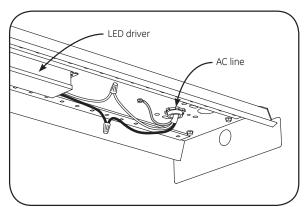
Install listed electrical fittings in the knockout holes for wire protection. Connect the AC line to the black (line) and white (neutral) input wires of the LED driver using 18-14WG twist-on wire connectors. Connect the green (ground) wire to the ground screw of the housing.
