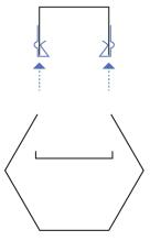
1: Attach clips to fixture body
