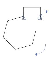
5: Slightly pry clips on one side and pull wire guard up and out to hinge. This is mainly for maintenance... it's not part of installation.
