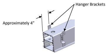
Smaller gap side of Bracket for 9/16" lay-in grid
