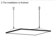
Note: 2\*2ft: 2 pcs suspension kits needed for installation. 1\*4ft: 3pcs supsention kits needed for installation.
