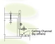
Mounting method when fixture is supported by perimeter ceiling structure. Ceiling channel by others.
