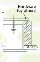
Mounting method when fixture is supported in a wood frame construction.
