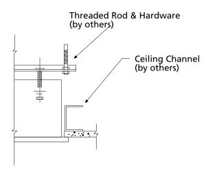
Mounting method when independent support of fixture is required. Threaded rod and ceiling channels by others.
