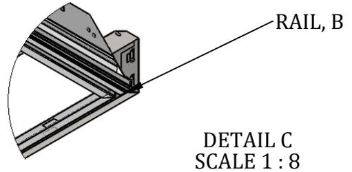
1. SLIDE FIXTURE INTO SHROUD ON "RAIL B", SHOWN IN "DETAIL C".
