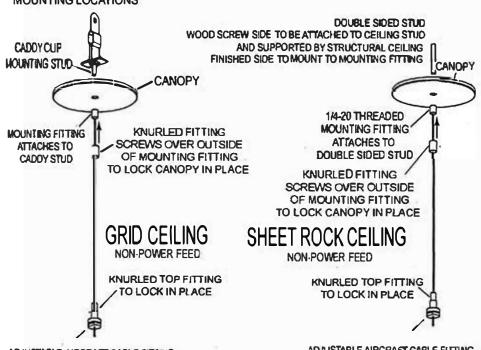
ADJUSTABLE AIRCRAFT CABLE FITTING TO BE INSTALLED TO FIXTURE AND SECURED IN PLACE WITH KNURLED TOP FITTING OR LOCKNUT ADJUSTABLE AIRCRAFT CABLE FITTING TO BE INSTALLED TO FIXTURE AND SECURED IN PLACE WITH KNURLED TOP FITTING OR LOCKNUT
