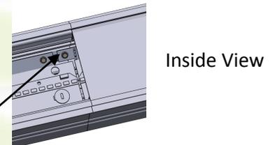
Fasten extended reflector tabs to joining fixture.
