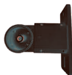
N2FWP-SFARM2-D SFARM2 Mount An optional cast aluminum mast arm adapter secures fixture head to nominal 2"(2-3/8" O.D. pipe size) horizontal steel tenon arm.
