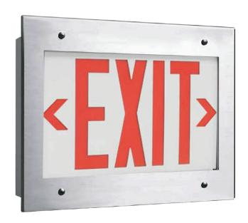
OUR **CLIR** is completely sealed recessed exit sign enclosure featuring a onepiece seam welded housing and one-piece seam welded overlapping doorframe. Internal battery provides a minimum of 90 minutes emergency illumination. Developed for applications such as clean rooms, high tech manufacturing facilities, laboratories, hospitals, food processing facilities, and commercial kitchens.
