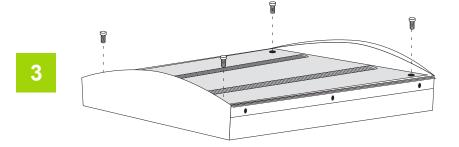
Remove 4 each #8-32 Phillips head screws from Reflector Tray.
