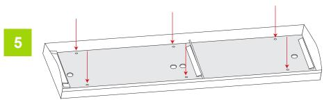
Drill pilot holes in desired mounting surface (usually over an electrical junction box that will be used to power fixture). Use appropriate fasteners/anchors (supplied by others) for the fixture weight as well as mounting surface.
