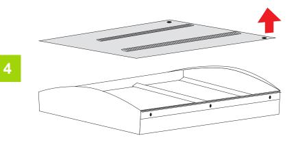
Remove Reflector Tray using caution to **not place strain on LED wiring**. This will expose 6 each 3/8" mounting holes for surface mounting application. Hardware supplied by end user for mounting.
